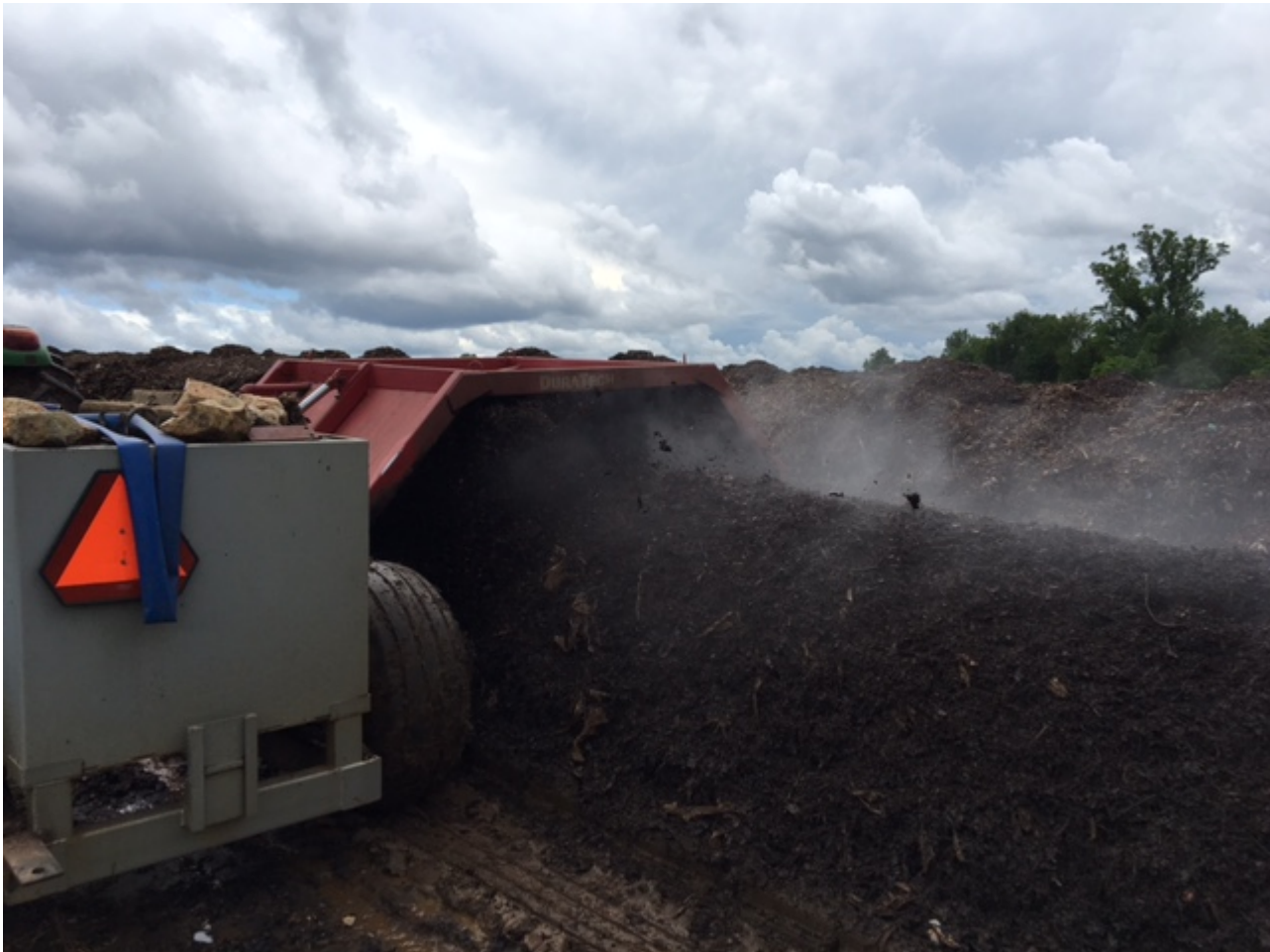
Commercial compost operation using rotating aerator windrow. Note the “younger” row of compost materials in the background. Photo: Ralph Morini
