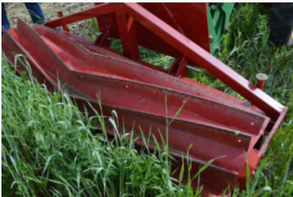
Roller crimper on cover crop Photo: NRCS Oregon
